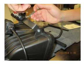
Now tighten the nuts firmly by holding the head end of the screw against it again and tighten the nuts.
