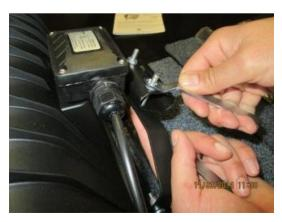
Now loosen the two protruding screws on the lower part of the spotlight to remove the oval guide.
