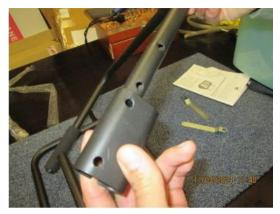
Now put the oval guide over the retaining bracket until the holes are on top of each other. In the picture, this is further to the right.
