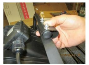
Here we now see the retaining bracket with the oval guide at the bottom of the spotlight with the two screws going through all the parts.
