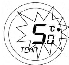
Use the Touch Ring to set the preferred temperature and confirm the choice using the OK button. Once the temperature setting is confirmed, the HOLIDAY mode will be activated. While in this mode the HOLIDAY mode indicator
