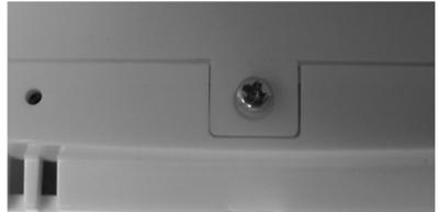
After undoing the screw pull it forward until the screw stops moving, then carefully separate the two halves of the case by gently pulling in an upwards direction. Once the case has been separated, the batteries should be visible:
