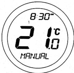
When the ST620 is operating in Manual Override mode, the LCD will display MANUAL instead of AUTO. The manual setting will remain in effect until the next programme time is reached, programme or clock settings are changed, an operating mode change is detected or the Manual Override mode is cancelled.
