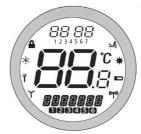
The display consists of a combination of symbols and alphanumeric displays. The top row is a time and day of the week indicator, the centre row is used to indicate temperature (in Celsius), and the bottom row is an alphanumeric display for menu and status messages. The symbols around the outside of the display are status indicators — an explanation of what these indicators mean is shown below.
