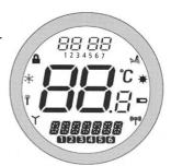
After 2 seconds the ST620 will then operate in NORMAL mode and display the current room temperature, with the RCC indicator flashing.
