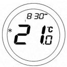
To turn off FROST mode, select the FROST menu and then by using the Touch Ring scroll to the OFF setting. Press the OK key to confirm the setting.
