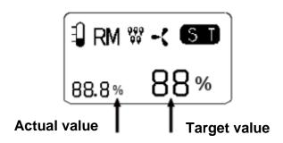
2. as the target value is reached, the unit switches off and the LED light changes from green to red.
